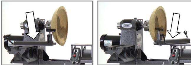
Move the gap section to the headstock and turn up to 32" diameter. Move the banjo and toolrest to either side of the work.
