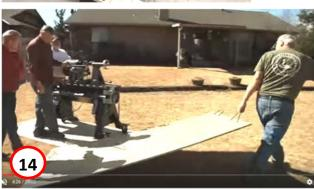
14) If you need to move your lathe across the yard or unpaved driveway, you can use the sides of the crate to make a temporary road way. In this picture, the crew has installed the Robust caster set. You can also use a pallet jack, or appliance dollies (be sure to secure them to the lathe). Again, go slow.
