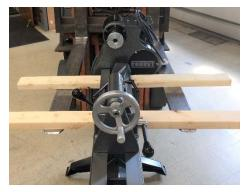
You can lift the S16 by putting 2x4s under the ways. 3-4 people can usually move the lathe fully assembled this way. Be sure to place one of the 2x4s as close to the headstock as possible, this is where most of the weight is.
