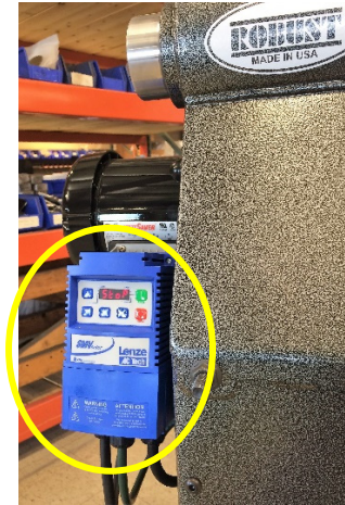
VFD (aka “inverter”) located on the side of the headstock
