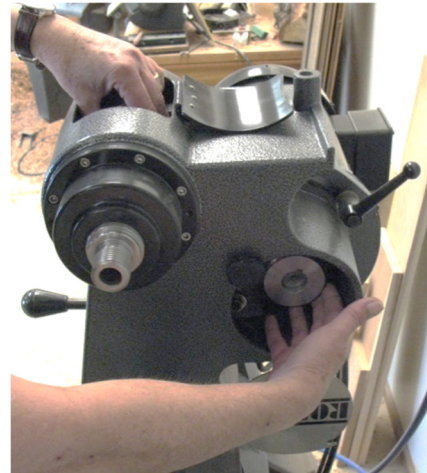
High speed is on the left, low speed/high torque is on the right (where belt is now)
