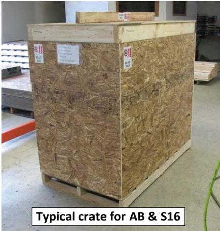
The American Beauty and Sweet 16 are shipped fully assembled, bolted to a skid and protected by a full wooden crate. Dimensions for the standard bed AB and short and standard bed S16 are 61" long, 36" wide and 62" high. Depending on model and options, the total weight is 600-950 lbs. Long bed crates are 85" x 36" x 62" and will weigh 700 to 1100 lbs.
