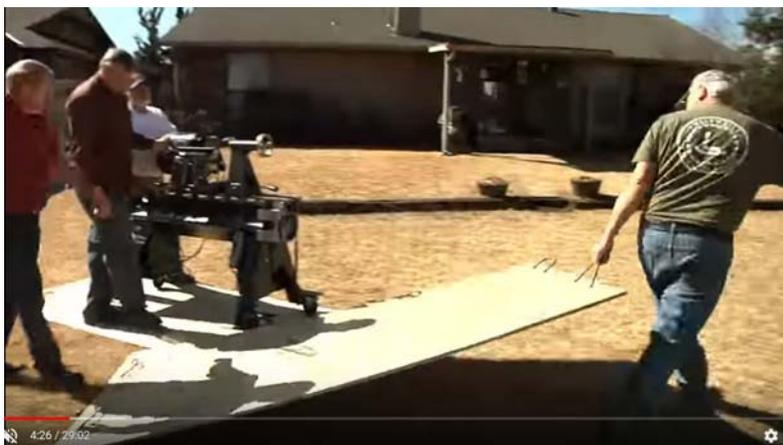
This group is using the caster set to move the lathe into a back yard workshop. They are using a couple of pieces of plywood for a temporary roadway across the lawn. The sides of shipping crate can be used for the same purpose.
