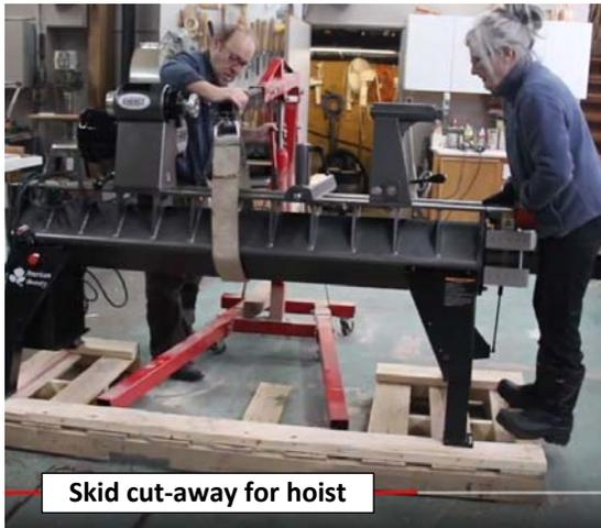
The lathe is held to the skid with four bolts. After removing the nuts from the bolts, these new owners are using an engine hoist to remove the lathe from the skid. One is managing the hoist and the other is guiding the lathe. Note how they have cut away the skid to get the engine hoist under the lathe.
