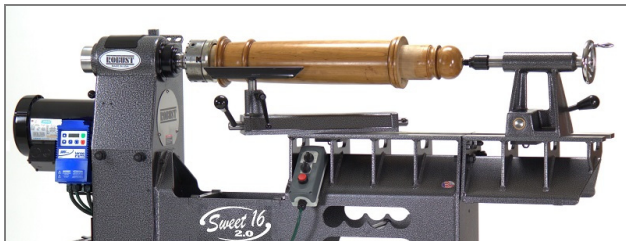
Position the gap at the end of the bed to turn long spindles. Note: the banjo bridges the gap.
