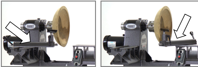
Above: Move the gap section to the headstock and turn up to 32" diameter. Move the banjo and toolrest to either side of the work.
